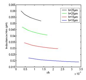
Fig.2 The inductance depending on the length of the metallic nanotube
